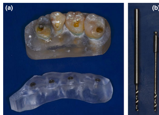
Figure 1 A test block with 4 resin embedded teeth (a, top) and the matching guide rail (a, bottom). With the guide in place, the entrance has been marked and enamel and filling material was cut with a high-speed bur exposing the entrance of the simulated access cavity. A commercially available twist bur with a diameter of 1.2 mm (b, left) and the same bur modified to be used through the guide sleeve (b, right).
